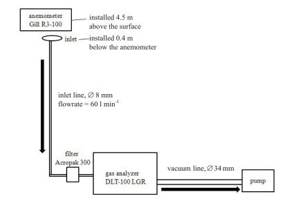
Fig. 2. Scheme of the eddy covariance system for measuring methane. The arrows indicate the direction of the intake air.
